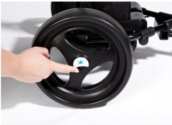
To check that the wheel is properly in position pull on the wheel. If it is properly in position it will not move.
